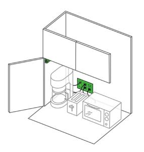
Docking Drawer's Safety Interlock Disconnect with Corner Mount Limit Switch is designed to be used in both 15 and 20 amp applications. The Safety Interlock Disconnect with Corner Mount Limit Switch can be wired in series with up to 2 receptacles\* and can de-energize up to four devices or appliances at one time, when the cabinet door is closed. ETL Listed to UL 498 and CSA 22.2 #42 and approved for use in the US & Canada\*\*. Possible applications include:
