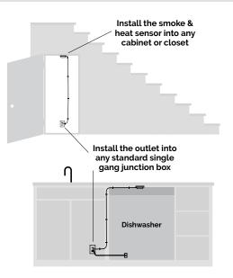
Ex: Connect your dishwasher to the outlet, and locate the smoke and heat sensor between the dishwasher and countertop. Docking Drawer's 20 amp Fire Guard Outlet is a single gang electrical outlet featuring one NEMA 5-20 receptacle and one interlock switch connector, as well as a smoke and heat sensing unit. The smoke & heat sensor mounts inside enclosed spaces to de-energize the outlet if smoke or heat is detected. Possible applications include:
