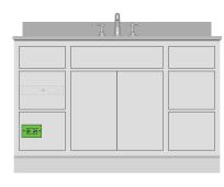
*Do NOT put the electrical* supply directly behind the drawer box as it may *interfere with the cable* management arms
