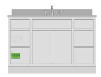
Do NOT put the electrical supply directly behind the drawer box as it may interfere with the cable management arms
