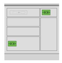
Do NOT put the electrical supply directly behind the drawer box as it may interfere with the cable management arms
