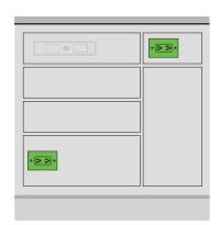
*Do NOT put the electrical* supply directly behind the drawer box as it may *interfere with the cable* management arms
