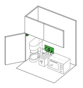
Docking Drawer's Safety Interlock Disconnect Kit with Corner Mount Limit Switch enhances the safety of stationary kitchen appliance garages by de-energizing the power outlet and up to 4 connected devices whenever the cabinet door is closed. This safety outlet can be wired in-series with the included receptacles, featuring (4) 20amp AC ports. ETL Listed to UL 498 and CSA 22.2 #42 and approved for use in the US & Canada\*. Possible applications include:
