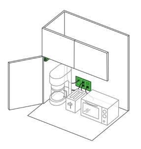
Docking Drawer's Safety Interlock Disconnect Kit with Corner Mount Limit Switch enhances the safety of stationary kitchen appliance garages by de-energizing the power outlet and up to 4 connected devices whenever the cabinet door is closed. This safety outlet can be wired in-series with the included receptacles, featuring (2) GFCI and (2) 20amp AC ports. ETL Listed to UL 498 and CSA 22.2 #42 and approved for use in the US & Canada\*. Possible applications include:
