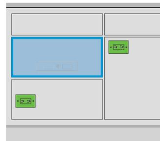
*Do NOT put the electrical supply directly behind the drawer box as it may interfere with the cable management arms*
