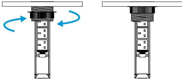
**Step 5 -** Connect the power cord to a power source within 1.5m, ensuring the outlet can open and close without tension on the cord.
