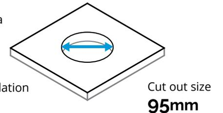
**Step 3 -** Rotate the adjustable ring in a counter-clockwise direction to remove. Place the power cord through the installation cutout and then insert the base of the outlet into the cut out. Be careful to avoid damage to power cord.
