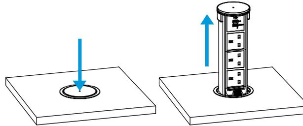
**To Close -** Press the "Push to Release" button to partially retract the outlet. Then press the top of the outlet to push the rest of the tower into the worktop and to lock into place.
