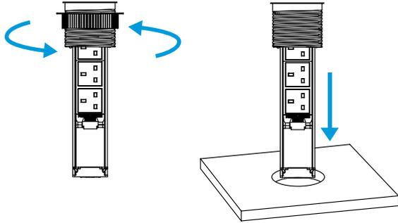
**Step 4 -** Adjust the front of the product to face the desired direction. Under the worktop, rotate the adjustable ring in a clockwise direction to tighten. Note that when the adjustable ring is askew, it will get stuck. If this occurs, re-tighten after alignment.
