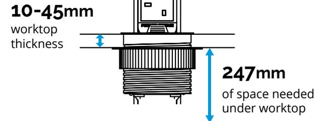
**Step 2 -** Cut a 95mm hole in the surface of the worktop to create the installation cut out.
