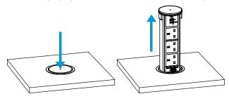
**To Close** - Press the "Push to Release" button to partially retract the outlet. Then press the top of the outlet to push the rest of the tower into the worktop and to lock into place.
