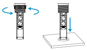
**Step 4** - Adjust the front of the product to face the desired direction. Under the worktop, rotate the adjustable ring in a clockwise direction to tighten. Note that when the adjustable ring is askew, it will get stuck. If this occurs, re-tighten after alignment.
