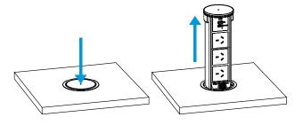
**To Close -** Press the "Push to Release" button to partially retract the outlet. Then press the top of the outlet to push the rest of the tower into the benchtop and to lock into place.
