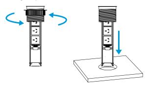
**Step 4** - Adjust the front of the product to face the desired direction. Under the benchtop, rotate the adjustable ring in a clockwise direction to tighten. Note that when the adjustable ring is askew, it will get stuck. If this occurs, re-tighten after alignment.
